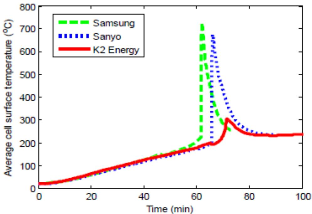
*The battery cell surface temperature during external heating (oven) abuse test, showing the temperature rise upon external heating and the rapid temperature peak due to thermal runaway for two types of cobalt based cells (Samsung and Sanyo) and for a lithium iron phosphate cell (K2 Energy). All three cells are of the 18650 type. Reprinted with permission of F. Larsson [3].*
